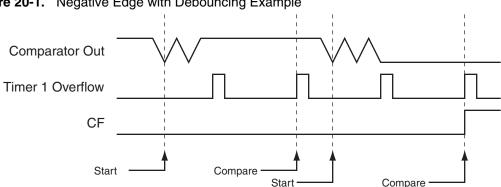
Figure 20-1. Negative Edge with Debouncing Example
