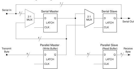
Figure 19-3. SPI Shift Register Diagram
