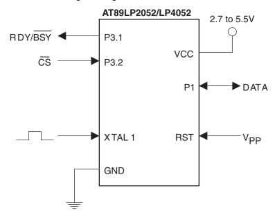
Note: Sampling of pin P3.1 (RDY/BSY) is optional. During Parallel Programming, P3.1 will be pulled low while the device is busy. Note that it does not require an external passive pull-up to V<sub>CC</sub>.
