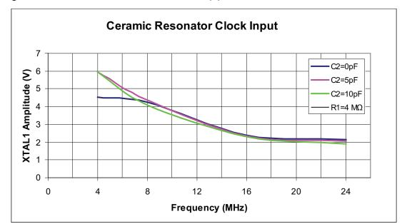
Figure 11-5. Ceramic Resonator Clock Source (B)
