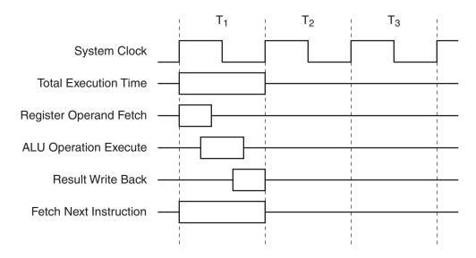
Figure 8-3. Two-Cycle ALU Operation (Example: ADD A, #data)
