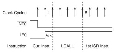
Figure 14-2. Maximum Interrupt Response Time
