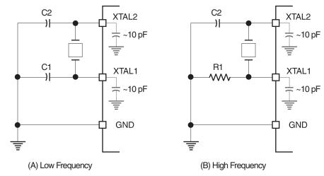
Note: C1, C2 = 0–10 pF for Crystals = 0–10 pF for Ceramic Resonators R1 = 4–5  $M\Omega$
