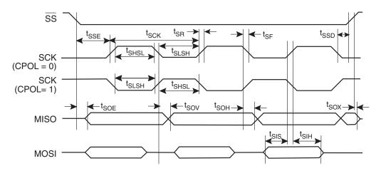
Figure 24-3. SPI Master Timing (CPHA = 1)
