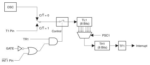
Mode 0 operation is the same for Timer 0 as for Timer 1, except that TR0, TF0 and INTO replace the corresponding Timer 1 signals in Figure 16-1. There are two different GATE bits, one for Timer 1 (TMOD.7) and one for Timer 0 (TMOD.3).
