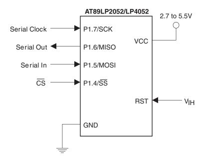
Note: SCK frequency should be less than 5 MHz.
