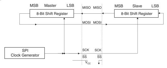
Figure 19-2. SPI Block Diagram
